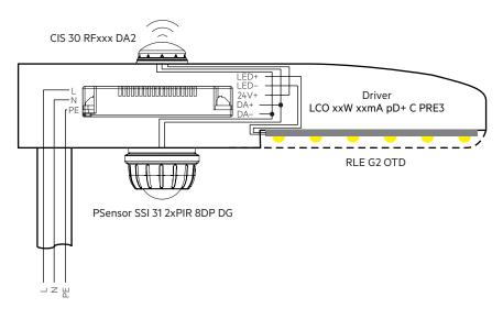
The sensor supports the Zhaga connectivity standard for Plug and Play luminaire extensions. This allows a toolless and flexible integration in luminaires. The connection interface is designed according to Zhaga Book 18 Ed. 3.
