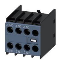
auxiliary switch, on the front, 3 NC, .1/.2, .1/.2, .1/.2, .-/--, current path: 1 NC, 1 NC, 1 NC, --, screw terminal, for contactors 3RT2 and contactor relays 3RH2
