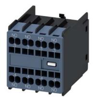
auxiliary switch, on the front, 4 NO, .3/.4, .3/.4, .3/.4, .3/.4, current path: 1 NO, 1 NO, 1 NO, 1 NO, spring-loaded terminal, for contactors 3RT2 and contactor relays 3RH2
