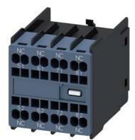
auxiliary switch, on the front, 4 NC, 51/52, 61/62, 71/72, 81/82, current path: 1 NC, 1 NC, 1 NC, 1 NC, spring-loaded terminal, physically coded, only with contactor relays 3RH2140 and 3RH2440 combinable (according to EN 50011)
