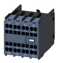
auxiliary switch, on the front, 3 NO + 1 NC, 53/54, 61/62, 73/74, 83/84, current path: 1 NO, 1 NC, 1 NO, 1 NO, spring-loaded terminal, physically coded, only with contactor relays 3RH2140 and 3RH2440 combinable (according to EN 50011)
