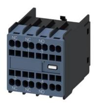
auxiliary switch, on the front, 1 NO + 2 NC, .1/.2, .1/.2, .3/.4, --/--, current path: 1 NC, 1 NC, 1 NO, --, spring-loaded terminal, for contactors 3RT2 and contactor relays 3RH2
