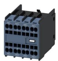
auxiliary switch, on the front, 3 NO + 1 NC, .1/.2, .3/.4, .3/.4, .3/.4, current path: 1 NC, 1 NO, 1 NO, 1 NO spring-loaded terminal, for contactors 3RT2 and contactor relays 3RH2
