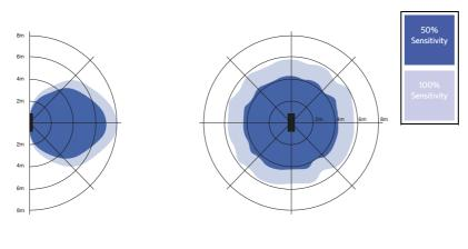
Installation - Wall mounted Suggested installation height 1-3m Installation - Ceiling mounted Suggested installation height 2.5-6m
